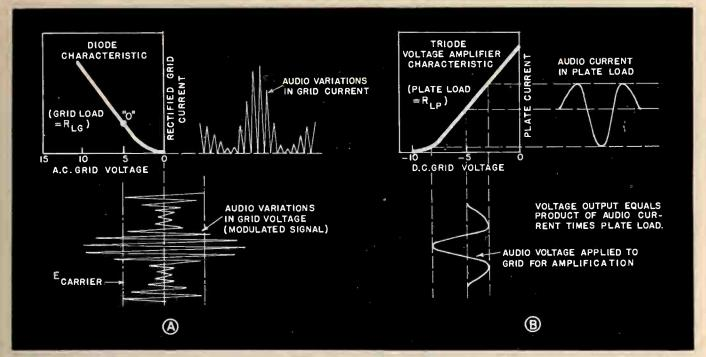
Fig. 2—Valve action of the rectifier portion of the grid leak detector removes the negative portions of the modulation cycles. The curved portion of the dynamic characteristic introduces distortion in the grid current. The audio triode characteristics in part B, show that distortion is least when grid bias is such as to keep signal voltage variations on the straight portion of the curve.
