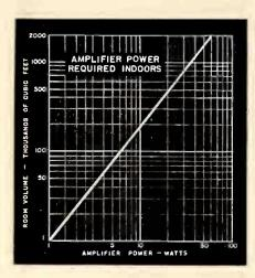
Fig. 1—Audio power requirements vary with initial noise level in the area. This graph is based on average conditions with a medium or low noise intensity.
