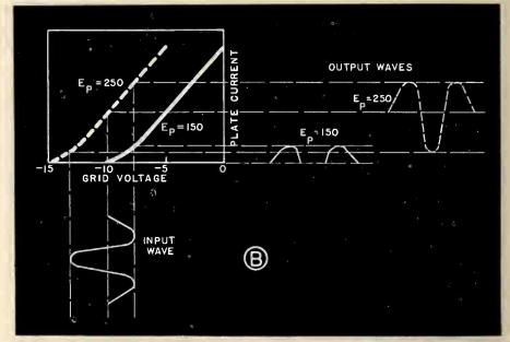
Fig 3B-Extreme distortion is introduced when bias is carried to cut-off. creasing the plate voltage moves the cut-off point further out on the grid voltage scale thus reducing distortion.
