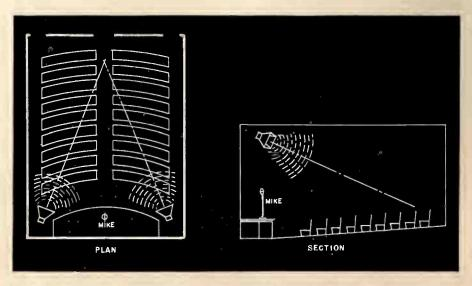
Fig. 2—Proper two-speaker lay out for best sound coverage and minimum of feedback. Note speakers mounted above and ahead of the microphone. Directional baffles put the sound where you need it.
