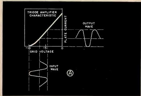
Fig. 3A—Increasing bias on grid has a neutralizing effect on the distortion introduced during detection.
